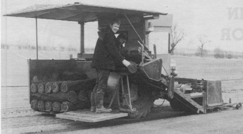
Turf is harvested by equipment that mows, cuts and rolls all in one go.
