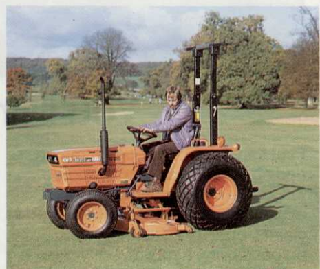
B8200—with a 3 cylinder, 19hp engine (and the option of hydrostatic transmission), this is the perfect machine for heavy duty work.
