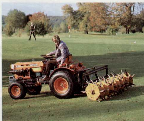
B7100HST—4 wheel drive has a powerful 16hp diesel engine, controlled by hydrostatic transmission, which includes creep speeds as standard.
