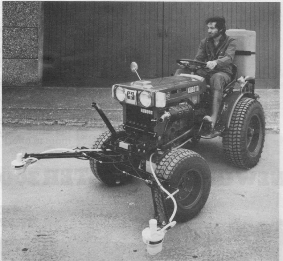
Chipman's twin-boom AccuRate mounted on a Kubota mini tractor.
