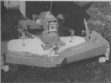
HINOMOWER ROTARY Front & Mid-Mounted 49 ins. cutting width
