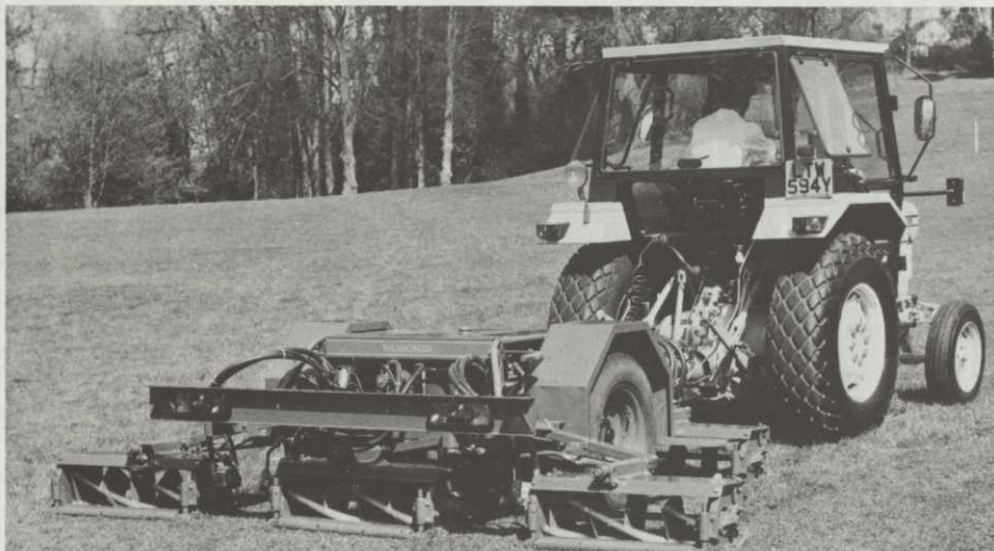
Ransomes' new five-unit hydraulic trailed gang mower can be hooked up to the tractor in under three minutes.
