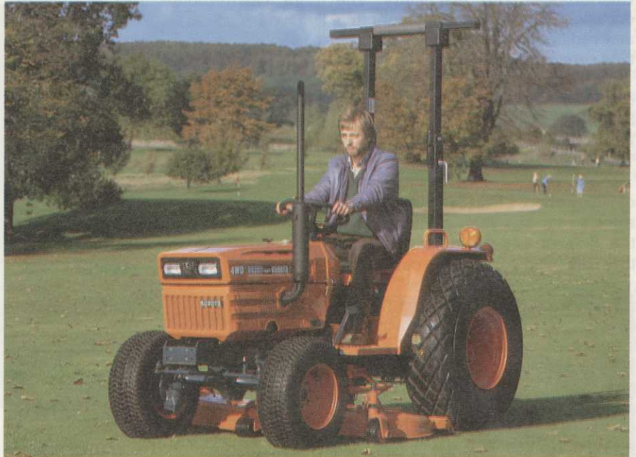
B8200 provides more power when you want it and where you want it. With a 3 cylinder, 19hp engine, it's ideal for the heavy work on course. Also available with hydrostatic transmission.
