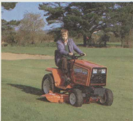
G3HST is the versatile ride-on, that makes short work of light rough. Highly manoeuvrable (thanks to hydrostatic transmission), 44" cutting width mid-mounted mower can cut almost anywhere, but always with miserly fuel consumption and minimal maintenance.
