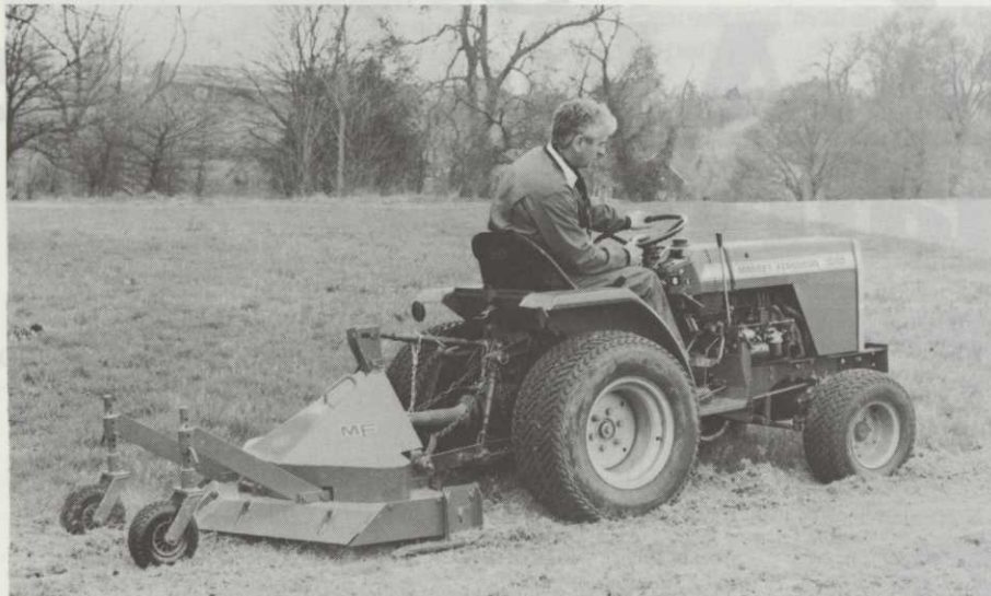
Massey-Ferguson is introducing a new range of versatile compact tractors to the UK. The MF 1010 produces 16 engine hp and is the smallest of the three new machines for which rear- or mid-mounted mowers will be available, as well as a wide range of other equipment including loaders, diggers and rotary cultivators.
