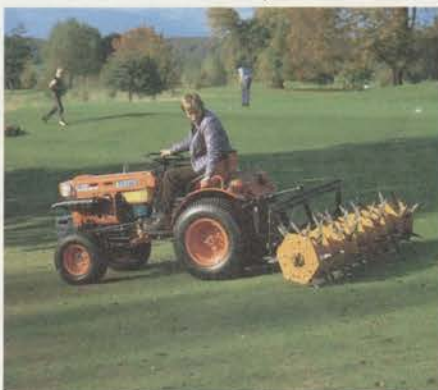
B7100HST has a powerful 16hp diesel engine, controlled by hydrostatic transmission, which includes creep speeds as standard. It will earn its keep all over the course.
