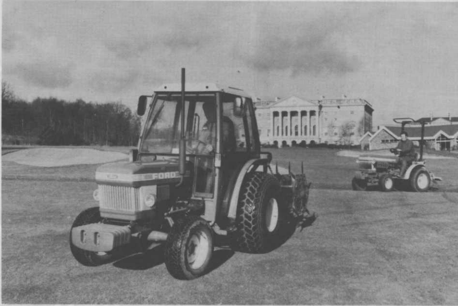
A 1910 Ford Compact tractor with turf splitter and a 1210 tractor with mole plough at Thorndon Park.
