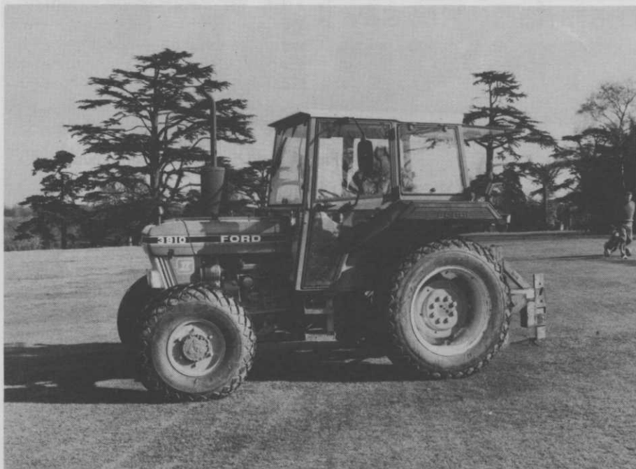
Ford's 3910 four-wheel drive tractor with turf tyres at work mole ploughing Dyrham Park fairways.
