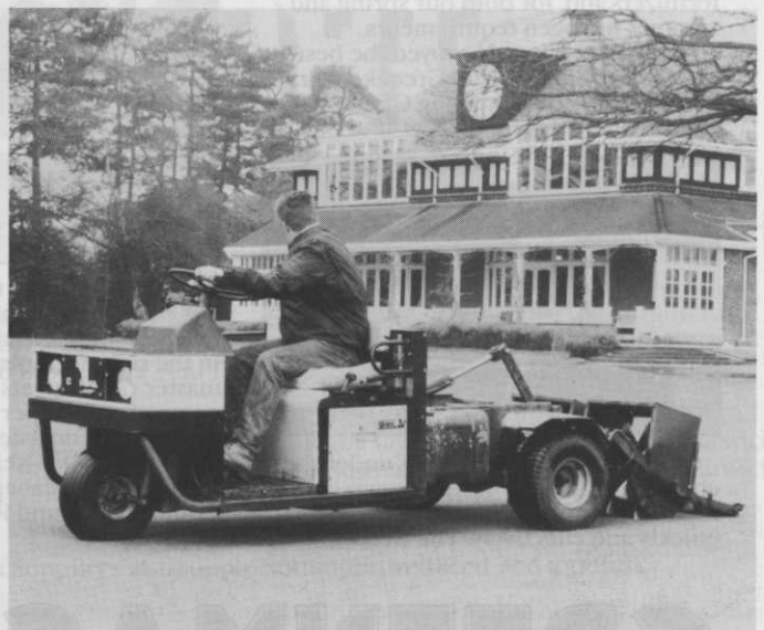
Cushman equipment slitting the Old Course 18th.
