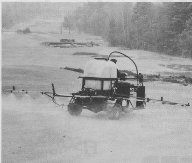
Mounted at the rear of a Cushman Turf Truckster, a 66-gallon Huxley sprayer.
