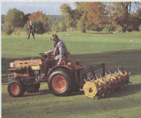
B7100HST—4 wheel drive has a powerful 16hp diesel engine, controlled by hydrostatic transmission, which includes creep speeds as standard.
