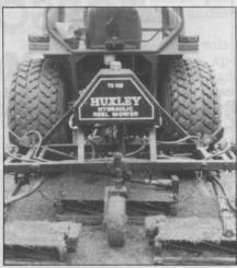
items give the mower the characteristics of a trailed unit in work, allowing the frame to follow ground contours independently of the tractor.
