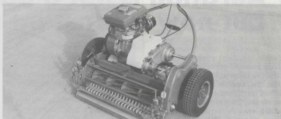
The Bunton 22in greens mower complete with powered rotary brush between the front roller and cutting reel.
