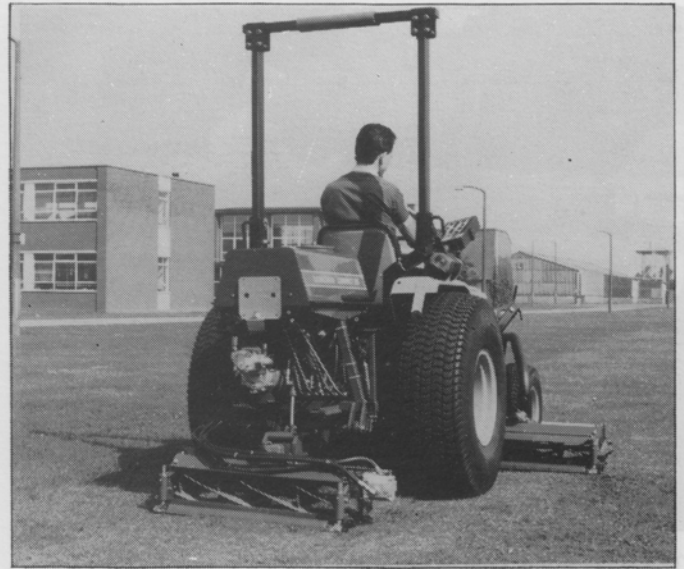
The new Ransomes Compact 215 mounted triple gang mower for use with tractors of around 18hp.
