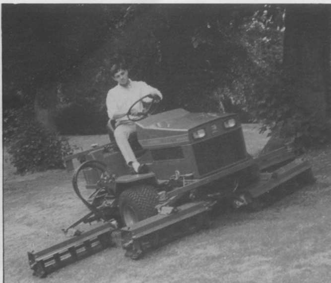
Differential lock and power steering have been added to the Ransomes Motor 3500.
