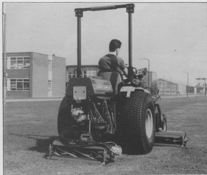
The new Ransomes Compact 215 mounted triple gang mower for use with tractors of around 18hp.
