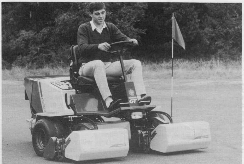
The new hydraulically operated GT triple greens mower.
