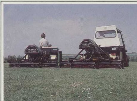
FINE TURF SCARIFIER (H44): Mounted on the Turf-Truckster's three-point linkage frame (H16), the pto-driven Huxley Fine Turf Scarifier has a 36in working width and 52 thin, double-edged blades to remove dead, matted and lateral-growing grasses. Front and rear adjustable rollers give precise control over scarifying depth (max. \frac{3}{4} in), blade spacing is variable (min. \frac{5}{16} in) and the grass box swings over for easy emptying.
