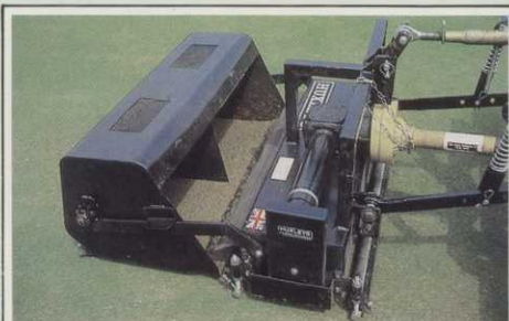
FINE TURF SCARIFIER (H44): Mounted on the Turf-Truckster's three-point linkage frame (H16), the pto-driven Huxley Fine Turf Scarifier has a 36in working width and 52 thin, double-edged blades to remove dead, matted and lateral-growing grasses. Front and rear adjustable rollers give precise control over scarifying depth (max. \frac{3}{4} in), blade spacing is variable (min. \frac{5}{16} in) and the grass box swings over for easy emptying.
