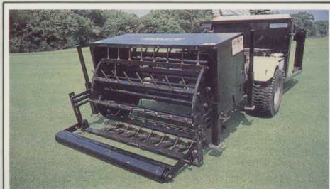
MULTI-TINE AERATOR (H34): With its 40in working width, the Huxley Multi-Tine Aerator is able to carry out a full range of aeration tasks. This attachment is available with a choice of 4in solid, 4in hollow or 3in slitting tines (see back page), and has a large diameter drum which helps produce a clean surface finish. The heavy rear roller smooths the surface after solid or slit tining. Raised, it adds weight for hollow coring.
