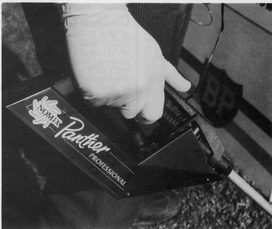
The speed regulator and its controls are built into the handle of the Nomix Panther lance together with a headphone socket.
