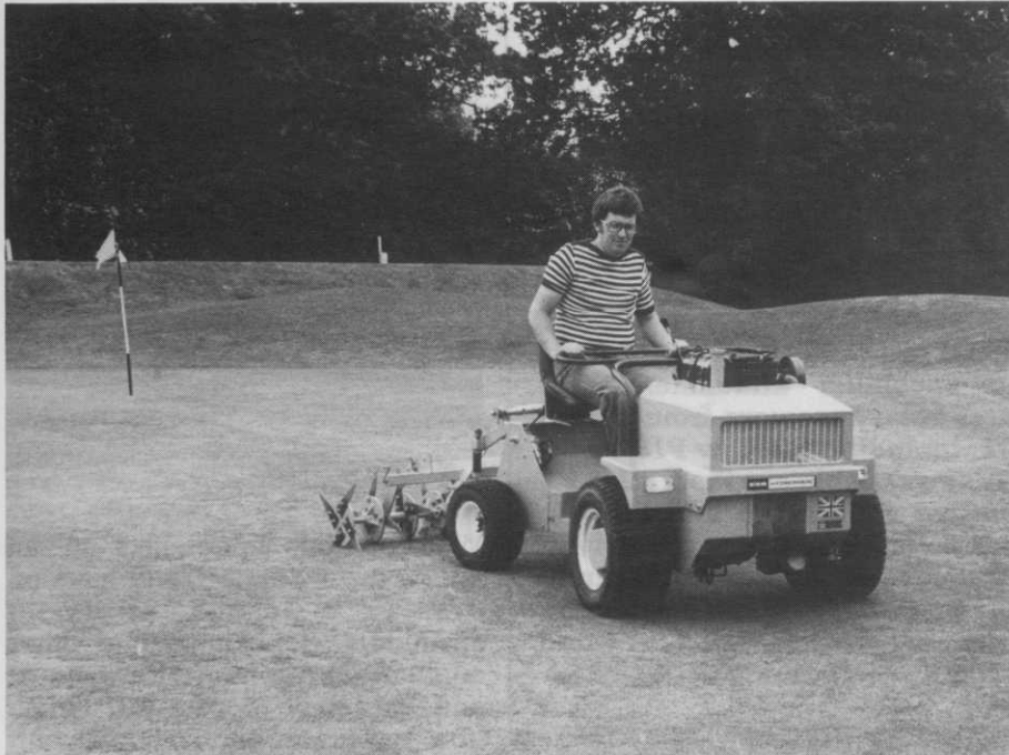
SISIS Hydromain Fourteen with deep-slitting aerator.
