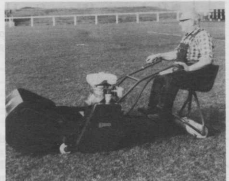
HYDROSTATIC GREENSMASTER 30 ins. & 36 ins. cutting width
