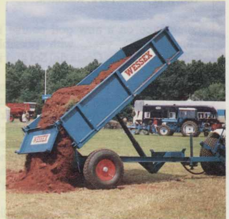
22cwt hydraulic tipping trailer
