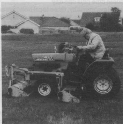
HINOMOWER 398 Hydraulic cylinder mower on C17 Hinomoto tractor
