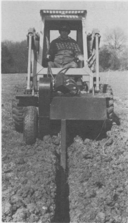
The Skid-Steer Trencher.
