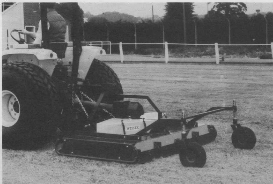
Suitable for tractors in the 30-50hp range, the Wessex P/18 professional rotary mower has a 6ft cutting width.
