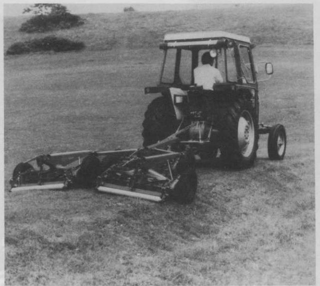
RANGER TRAILED & HY-RANGER MOUNTED GANGS 30 ins. & 42½ ins. gangs to give large choice of cutting widths
