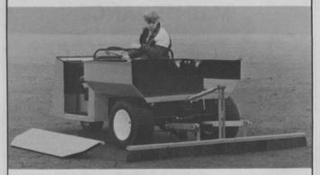
SOFT TURF TYRES SHORT TIPPING BODY LIVE-HYDRAULIC LIFTING AND TIPPING
