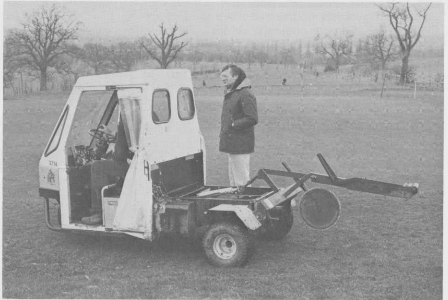
Norman Leddy, manager of parks and woodlands for the London borough of Hillingdon, stands beside a Cushman Three-Wheel Truckster at Harefield Place Golf Course, Uxbridge. Mounted on the rear hydraulic linkage is a variable-depth moleblade with turf-slicing disc coupler for relieving compaction and improving drainage on greens and surrounds.
