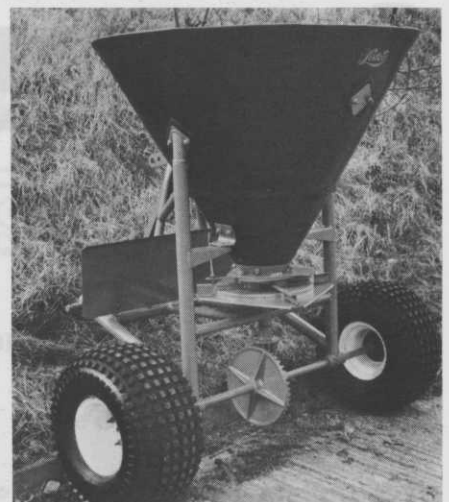
The new low ground pressure spreader.
