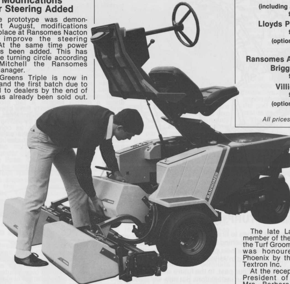
The operator's platform on Ransomes new all-hydraulic GT Triple Greens Mower can be raised in seconds for easy access to the centre cutting unit and to empty the grasscatcher.
