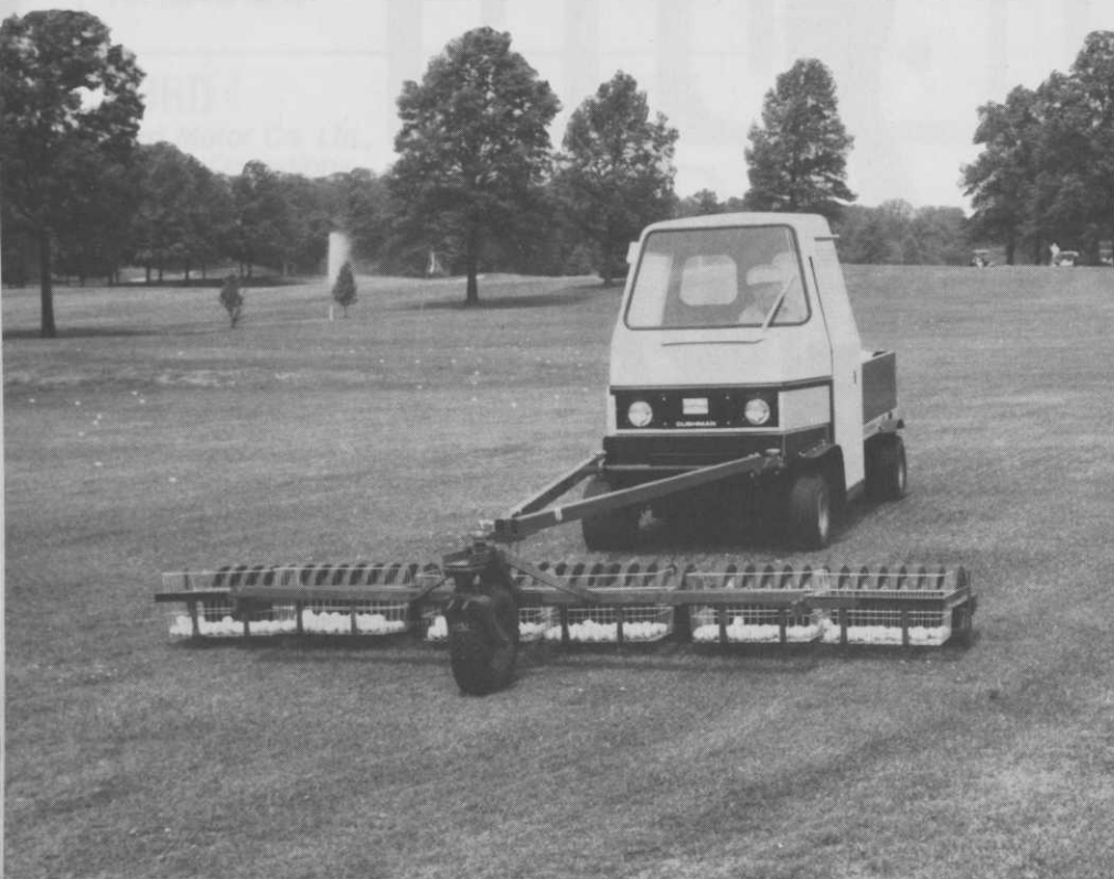
Grounds technician Bernie Johnson sweeps the Bellerive Country Club driving range with the club's unique front-mounted ball picker
