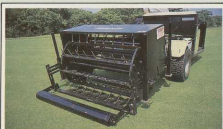
MULTI-TINE AERATOR (H34): With its 40in working width, the Huxley Multi-Tine Aerator is able to carry out a full range of aeration tasks. This attachment is available with a choice of 4in solid, 4in hollow or 3in slitting tines (see back page), and has a large diameter drum which helps produce a clean surface finish. The heavy rear roller smoothes the surface after solid or slit tining. Raised, it adds weight for hollow coring.
