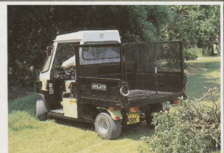
LONGBOX/FLATBED (H7): For maximum versatility, the hydraulically-tipped Longbox has quickly removable sides and tailgate enabling it to be used either as a flatbed or pick-up box transporter. Maximum payload is 1,500lbs and internal dimensions are 48in x 52in x 13in. Clip-on, mesh EXTENSION SIDES (H7a) – shown above right and on front cover – are available as an option to further extend this useful attachment's load-carrying ability.
