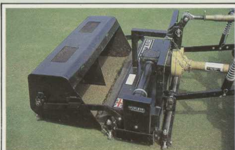
FINE TURF SCARIFIER (H44): Mounted on the Turf-Truckster's three-point linkage frame (H16), the pto-driven Huxley Fine Turf Scarifier has a 36in working width and 52 thin, double-edged blades to remove dead, matted and lateral-growing grasses. Front and rear adjustable rollers give precise control over scarifying depth (max. 3/4in), blade spacing is variable (min. 5/8in) and the grass box swings over for easy emptying.
