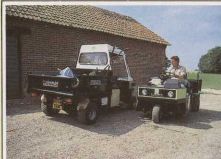
LONGBOX/FLATBED (H7): For maximum versatility, the hydraulically-tipped Longbox has quickly removable sides and tailgate enabling it to be used either as a flatbed or pick-up box transporter. Maximum payload is 1,500lbs and internal dimensions are 48in x 52in x 13in. Clip-on, mesh EXTENSION SIDES (H7a) – shown above right and on front cover – are available as an option to further extend this useful attachment's load-carrying ability.
