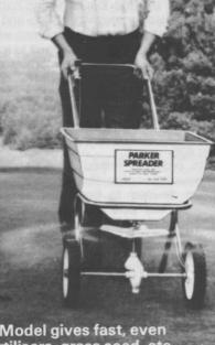
The Master Model gives fast, even distribution of fertilisers, grass seed, etc., providing a spread pattern of 5 feet feathering out to 8-10 feet. It has a unique sector control provided by a special stainless steel cut-off, enabling operator to spread to one side only. The hopper is corrosion resistant and holds sufficient fertiliser to treat one green without refilling.
