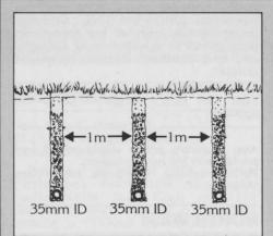
Use 35mm pipe at the required grade, with gravel fill and topped as required, for cost economy. Water will drain away horizontally only through pipe, not through gravel.
