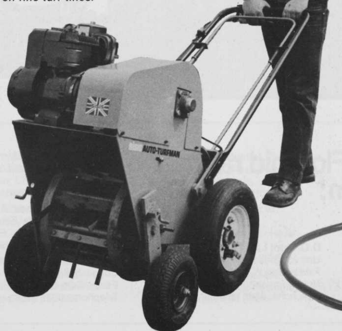
NEW SISIS Mk. 2 AUTO-TURFMAN Heavy duty, powered aerator for year-round use on fine turf tines.
