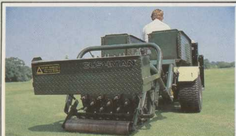
GREENSAVER AERATOR (C10): The Cushman Greensaver Aerator, with Weight Box set, is able to perform virtually all hollow coring (with core collection) and shallow aeration operations on fine turf. Three drum types are offered: standard 1/2in coring drum (shown here), with trap door for rapid core disposal; 3/8in coring drum, with trap door; and 2 1/2in deep slicing drum. All produce a 3 1/4in x 4in aeration pattern.
