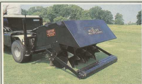
MULTI-DEPTH AERATOR (H84): Designed to carry out complete aeration treatment of all fine turf areas, the 42in wide Huxley Multi-Depth Aerator can be set to work from 4 1/2in to 9 1/4in deep to suit most aerating needs. Adjustable rear roller and a choice of three blade sizes (see back page) enable quick variation of working depth. Can also be used as a light roller only.
