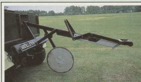
MOLEBLADE (H35): Hydraulically-controlled from the driver's seat, the Huxley Moleblade is able to relieve compaction and improve drainage/soil aeration in all problem turf areas. Working depth is adjustable in 2in steps down to 9in and the leading disc coupler and spring-tensioned rear roller ensure minimal turf tear and disturbance. A Weight Box Set (H26) – supplied with the C10 Greensaver – is needed for this attachment.
