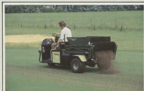
TOP DRESSER (C5): Mounted on the Turf-Truckster's chassis and driven by the power take-off, the Cushman Top Dresser produces a precise and even spread of most free-flowing materials across a 31 1/2in width. Capacity is 9 1/2 cu ft (approx. 1000lbs) and delivery is by a combination of belt conveyor and rotating nylon brush. Application rate is controlled by metering gate, with drive engaged/disengaged from the driver's seat.
