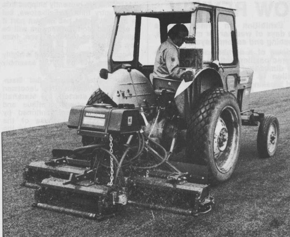
Pictured on a golf course fairway is Ransomes new Mounted 214 Verticut which has a working width of 7ft. and is suitable for use with tractors of 40hp and above.
