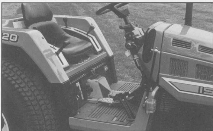
A stepthru deck of the Iseki TU Tractor gives the driver a much more relaxed place to operate.
