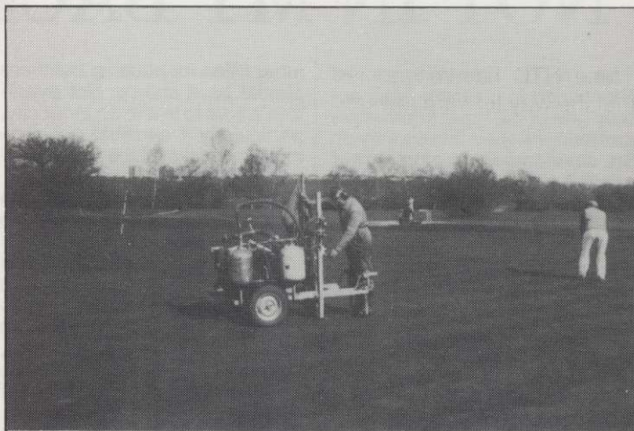
Play continues. The Terralift is shown treating a golf green whilst in play. Note lack of damage to the playing surface.
