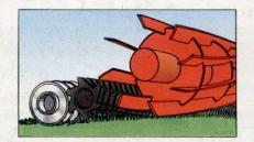
By cutting horizontal runners and removing thatch, the patented Turf Groomer attachment creates faster, truer and healthier greens without lowering height of cut.
