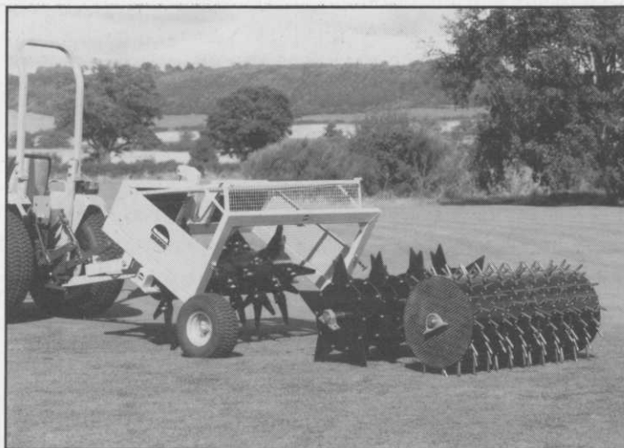
The new McConnel Dabro Interchangeable Ground Support System, consists of an Outfield Slitter, Green Slitter and Corer. All the implements slip easily in and out of the common frame.
