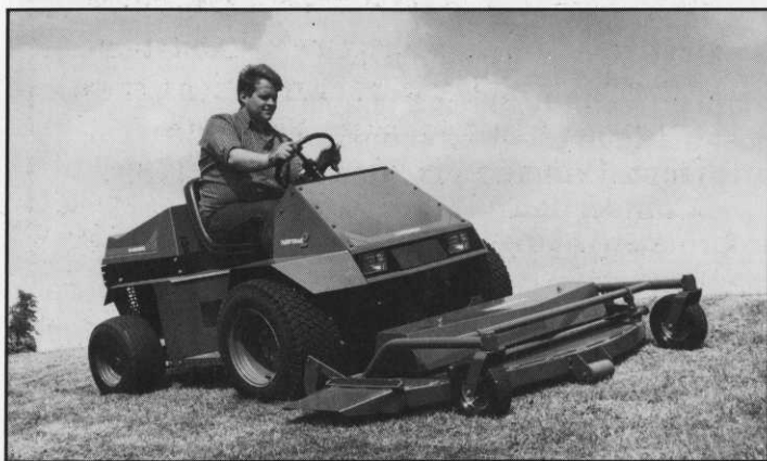
Ransomes new 16.5hp Kubota diesel engined TURFTRAK 2 power unit pictured at work with a front mounted rotary mower. The TURFTRAK 2 has an adjustable traction booster for transferring weight from the attachment.
