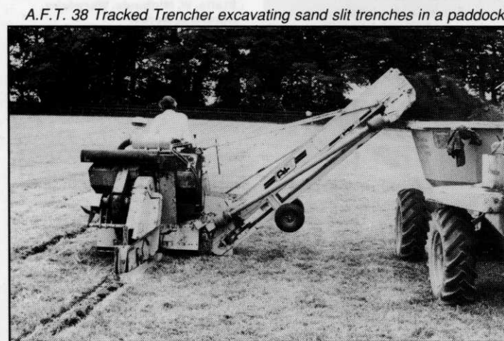
A.F.T. Wizz Wheel Trencher excavating for sand slits
