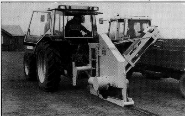
A.F.T. Wizz Wheel Trencher excavating for sand slits
