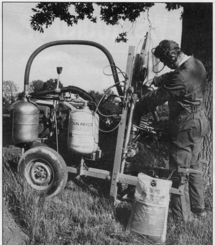
Colin Pryce pours a dose of fertiliser in the Terralift's canister before releasing a compressed air charge which will simultaneously shatter the soil in this oak's root zone and carry the fertiliser to the roots.
