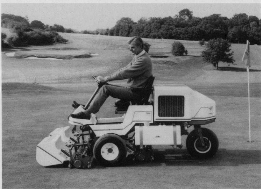
Huxleys new 358 Greensmower with optional hydraulics third wheel drive
