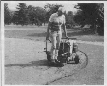
The Multicore Aerator with mini-tines hollow cores a badly thatched green
