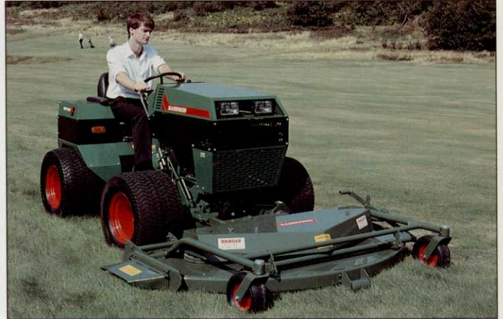
Turftrak 4 with three blade rotary mower
