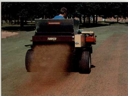
A high-speed rotating brush drives top dressing down into the turf.
