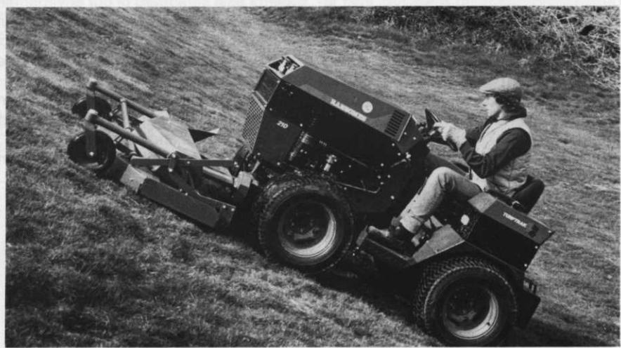
Adrian Archer cutting a tee bank with the Ransomes Turftrak
