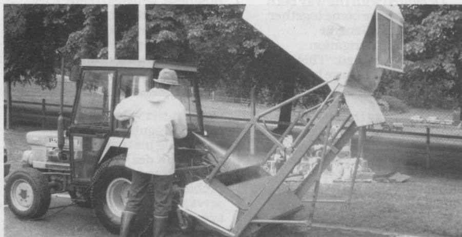
The Dynajet high pressure water cleaner in action
