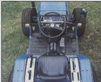
The Stepthru deck for even easier operation.
