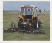
Ransomes Mounted Hydraulic 5 is a fullymounted, fine-cutting gang mower that's on fairways particularly effective undulations can make efficient mowing difficult. The five floating head, 6-knife cutting units produce a fine, ground-hugging cut of 3.43m. Finger-tip control raises the mower hydraulically and folds the outer units for ease of transport.
