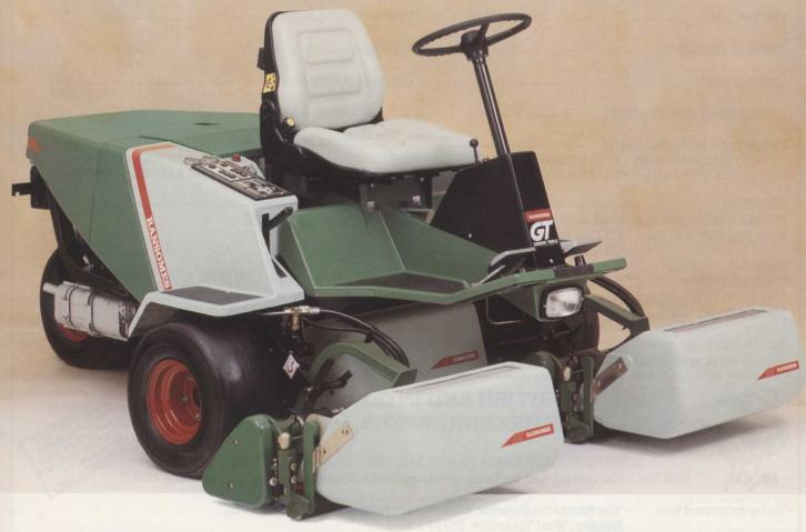
The new Ransomes GT is a revolutionary, allhydraulic triple greens mower with many unique features for precise control over all mowing operations. Its 9-knife cutting units are hydraulically driven and can be interchanged
