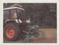
hydrostatic drive and single rear wheel steering. Wide front drive wheels and low centre of gravity give excellent traction and stability on slopes, with minimum turf compaction. Large capacity grasscatchers are also available.
