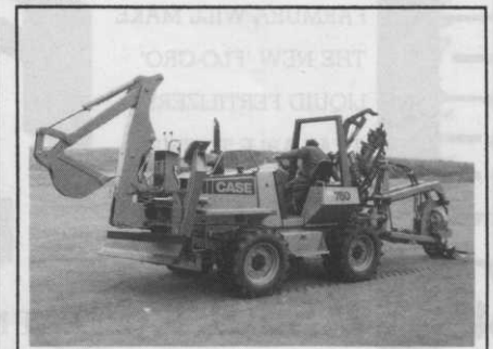
With four different attachments on the Case 760 'Quad' there is no need to hire-in additional machines for separate trenching functions.
