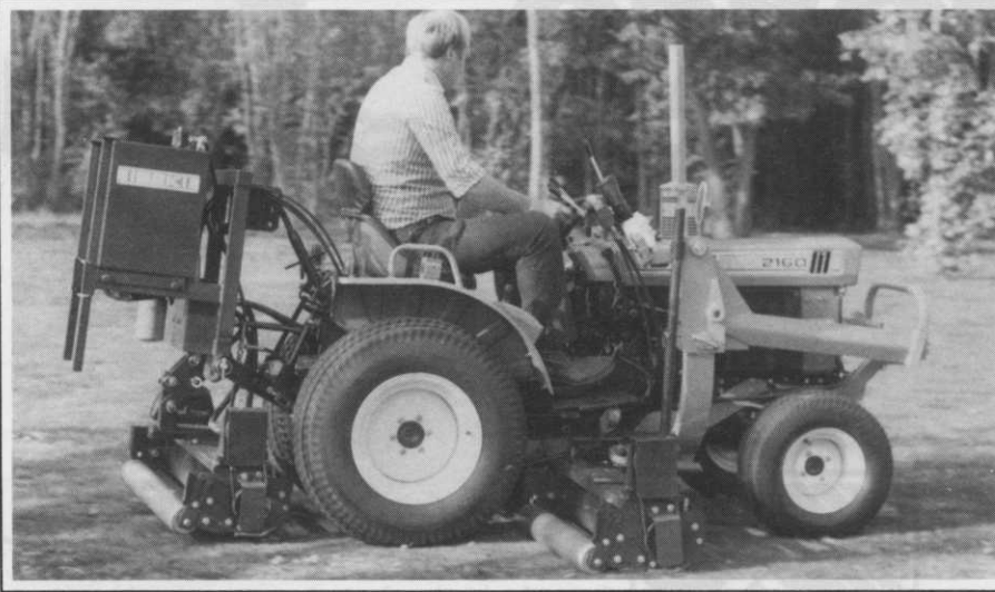
Iseki's TX Tractors are available with wrap around cylinder mowers for fairway or green surround moving
